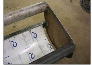
Dispenser assembly during construction
