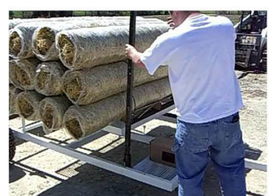
Put in the roll back stops
